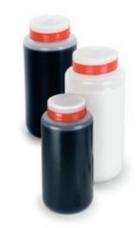
Series LVM-ML Marinelli beakers, for both HPGe and Nal(TI) detectors, are available in 500 mL, 1000 mL, 2000 mL and 4000 mL sizes. This configuration is useful where maximum efficiency is needed such as environmental samples. See below for a complete listing of available sizes.
