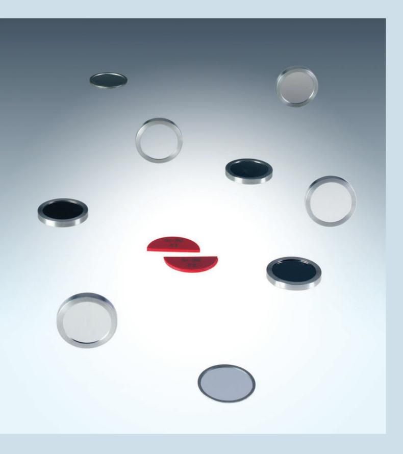
A wide range of beta emitting nuclides are offered for counting and educational uses. Certification of all BF Series sources includes both contained activity and  $2\pi$  emission rate. Sources are traceable to NIST with ±2% to ±5% accuracy at the 99% confidence level. Source configurations are surface conductive on all surfaces to enable their use in windowless proportional counters.
