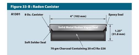
The EG-226C is supplied with 20 nCi (740 Bq) Ra-226 and is NIST traceable. Calibration accuracy is within  $\pm 5\%$  of the stated value at the 99% confidence level. Other activities and canister sizes are available on request.
