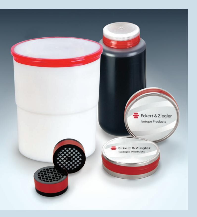
The model EG Series standards offer a convenient method to calibrate HPGe and NaI(TI) detectors for the analysis of soil and water samples, reactor coolants, air samples, and other environmental materials. Standard activity is 0.1 µCi (3.7 kBq) - 5 µCi (185 kBq). Customer supplied containers will be filled upon request.
