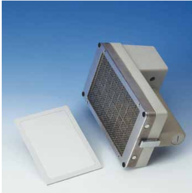
This picture shows the isotrak contamination monitor.
