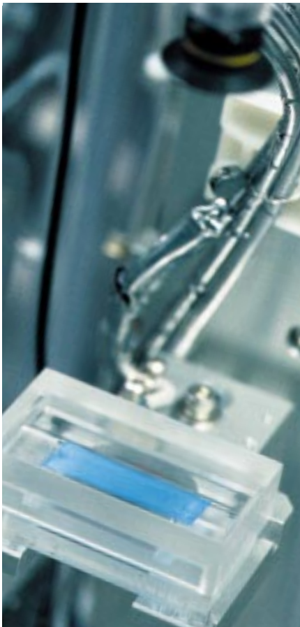
Production unit for balloon catheter radioactive coating
