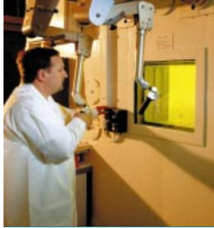
Hot cell for storing radioactive substances
